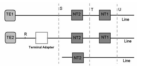
For large businesses it is common to have more telephone conversations going on simultaneously than the bus can handle. Therefore, another device, NT2, called a PBX, connected to NT1 and providing the real interface for telephones, terminals and other equipment. An ISDN PBX is not very different from an ISDN switch.
